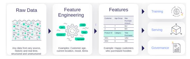
MLOps solutions should incorporate a feature store that defines the data collection and transformations just once for both batch and real-time scenarios, processes features automatically without manual involvement, and serves the features from a shared catalog to training, serving, and data governance applications. Feature stores must also extend beyond traditional analytics and enable advanced transformations on unstructured data and complex layouts.
