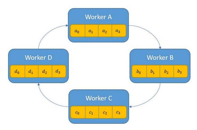
Horovod will run your code on all the given nodes (Specific node can be addressed via hvd.rank()) while using an hvd.DistributedOptimizer wrapper to run the synchronization cycles between the copies of your Neural Network running at each node.
